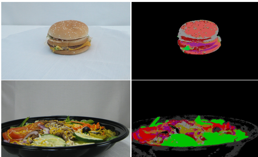
Figure 3. On the left are sample input pictures to the trained STF, and on the right are output visualizations shown such that each pixel is colored the color of the ingredient that it is most likely to be, according to our segmentation. In the Big Mac, the meat and lettuce are perfectly identified, and most of the bread was identified correctly. However, there is a fair amount of noise: part of the bun is labeled as bacon (purple). Clearly, these ingredient labels can be quite noisy, and any improvements in the ingredient labeling algorithm will cause corresponding improvements in this food recognition classifier.
